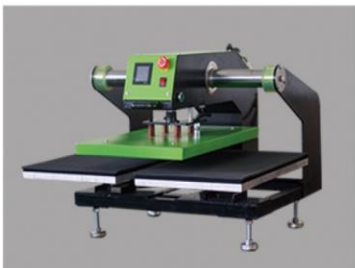
Model: FZLC-B2/Double Station Heat Press Plate size: 38x38cm/40x50cm/40x60cm Gross weight: 115 kg/127 kg/145 kg Features: Double station high efficiency, T-shirt threadable
