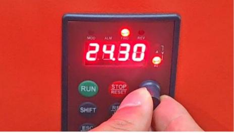
Use speed knob to adjust the moving speed of the bottom platens(**Do not make it higher than 25.00**)
